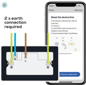
Follow the above diagram to wire the Smart Socket into the mains. The Socket should start to flash rapidly.
