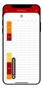
The scheduling can be selected as hourly increments on separate days. When you press the hour in any given day a temperature bar will be displayed.
