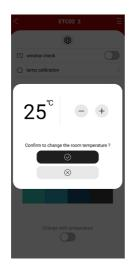
Use this function to manually adjust to the actual room temperature if it is not correct.
