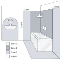
Suitable for indoor only. This product is rated as IP24. If the product is to be installed within a bathroom it can only be located within zone 3.
