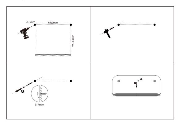
1) Drill holes on the wall according to the above instruction.
